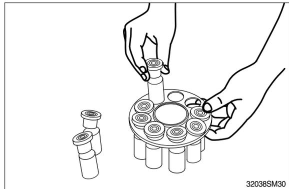
(10) Reassemble the piston assembly(121, 122) to the cylinder(111).
